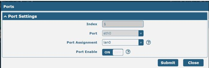
Note: R3000 Quad/R2110/R5020 does not support the "Port Enable" feature.
