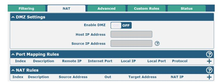
DMZ (Demilitarized Zone), also known as the demilitarized zone. It is a buffer between a non-secure system and a security system that is set up to solve the problem that users who access the external network cannot access the internal network server after the firewall is installed. A DMZ host is an intranet host where all ports are open to the specified address except the ports that are occupied and forwarded.
