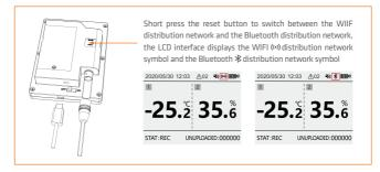
3) Follow the steps below to configure WiFi, the top of the screen displays " ", and the device has successfully configured WiFi;
