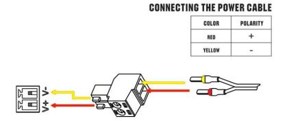
R1510 Router supports reverse polarity protection, but always refers to the figure above to connect the power adapter correctly. There are two cables associated with the power adapter. Following to the color of the head, connect the cable marked red to the positive pole through a terminal block, and connect the yellow one to the negative in the same way.
