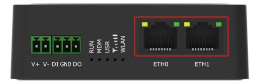
There are two Ethernet ports on R1510, including ETH0 (WAN/LAN), and ETH1. Each has two LED indicators. The yellow one is a link indicator but the green one doesn't mean anything. For details about status, see the table below.
