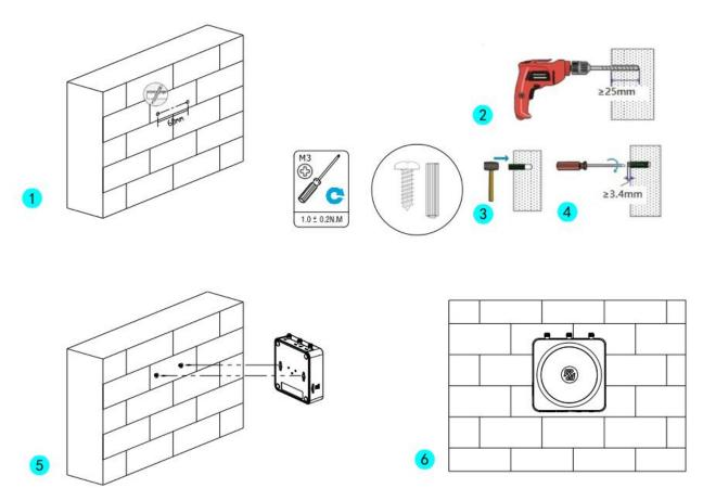
First, drill holes on the wall, the distance between the two holes is 60mm, then knock the expansion pipe into the wall with a rubber hammer, align the screw with the expansion pipe, insert the screw and reserve the corresponding length, and finally fix the product on the wall.
