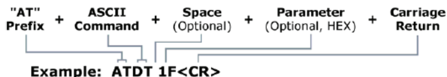
Figure 3.10. Syntax for sending AT Commands
