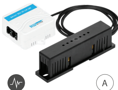
30A DC Current Probe 1W-UNI Current range: 0-30 A DC accuracy: \pm 2\%
