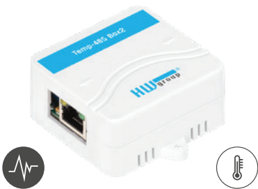
Temp-485 Box2 Temperature range: -10 to 70 °C, IP23 rating
