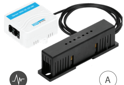
100A DC Current Probe 1W-UNI Current range: 0-100 ADC, accuracy: 2 %
