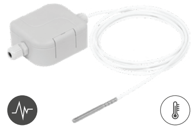
Temp-485-Pt100 Frost2 Temperature range: -190 to 150 °C, IP53 rating
