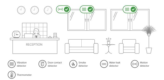
Water leaks or fires in hotels or house rentals can cause very costly damages. The SensDesk IoT portal helps you watch over all these risk factors. In case of an event it will immediately send out an alarm or react by shutting down water or activating a fire sprinkler. The SensDesk portal and HW group IoT devices have been successfully deployed in a number of solutions for many hotels and house rentals. ✓ Complex IoT monitoring
