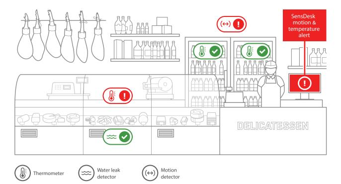
Storing food requires precise temperature monitoring, fast alarms and detailed reporting. SD devices with the SensDesk portal help you monitor your refrigerator temperature. The SD-WLD will detect water leaks under the refrigerator. Thanks to the SD-2xIn you receive alarms when unauthorized motion is detected in your store. All your data can be summarized in automated reports and emailed to you regularly.
