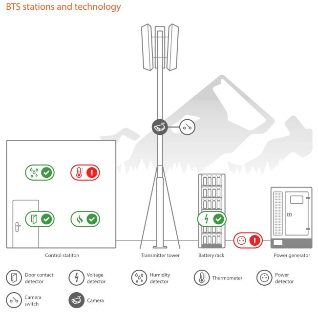
Remote technology needs reliable monitoring of cooling, heating, and site conditions. You may also need to monitor your proprietary technology using digital inputs and outputs. SensDesk and HW group IoT sensors can detect A/C failures, water leaks, movement, intrusion and more. SensDesk offers you different user and administration levels and tools for mass operations so it's robust and convenient even for large installations.
